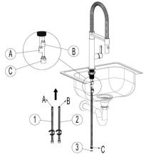
Connect supply hose(1)(2) into faucet,hot A and cold B. Connect shower hose C with washer (3) to C. Hand it.
