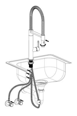
Check all connections at arrows for leaks. Re-tighten if necessary,but do not overtighten.
