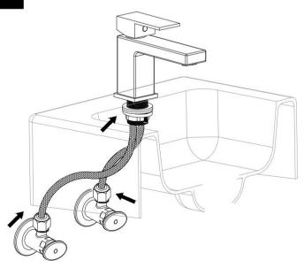
Open faucet and all way on , Check all connections at arrows for leaks. Re-tighten if necessary,but do not overtighten.
