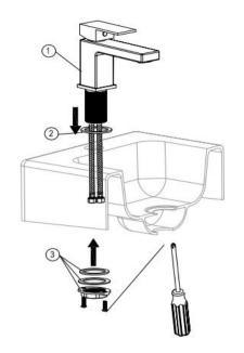
Position the faucet(1) onto sink, then tighten washer and lock nut(3) with screw.
